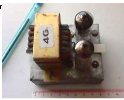
A simple QRP transceiver with full QSK for the CW sub-band of 40m. It uses two valves, a 6AQ 5
