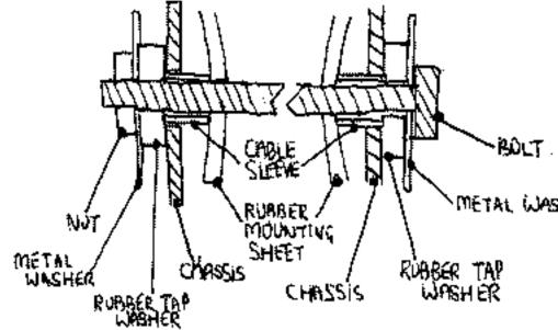
listen carefully for crackles and pops, look for smoke, and sniff for nasty smells. A few seconds after applying power I could detect the smell of burning rubber, and switched off before too much damage was done. Only one or two layers of the plastic tape wrapping the toroid had melted where in contact with the mounting bolt. I realised the cause of the heat almost immediately.
