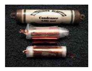
Here I attempt to make a capacitor out of kitchen foil and cling film, inspired by the work of H P Friedrichs (AC7ZL) and his book Voice of the Crystal". Eventually, I hope to build a whole CW transmitter with matching regenerative receiver, using entirely homemade components, including homemade valves. See AC7ZL's latest book
