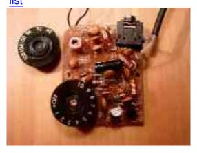
Last night I experimented with the 7088 cheap DC 40 m rx and found a simple way to get more audio output by using more of the internal circuitry of the chip. Now the audio level is just fine instead of being marginal.
