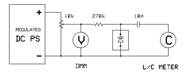
John VK6JY sends some results from Albany, Western Australia, obtained using the circuit shown here (right). The C-meter is an <u>AADE L/C meter</u> and the PSU is a 15V 20A DSE 3800 (overkill? What! Never).
