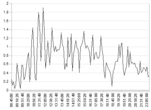
The datalogger text files can be loaded directly in Excel (etc) and the chart shown to the right is an example trace obtained during an overnight wind speed logging session.
