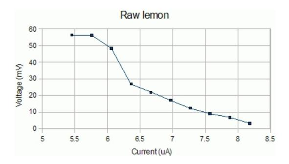
My first attempt at a lemon battery consisted of a standard lemon, fresh from the supermarket, with a copper wire (solid core household cable with the insulation stripped off) poked in one side and a normal steel bolt pushed in the other side. To test this power generation masterpiece, I rigged up a 10k variable resistor in series with a 330-ohm fixed resistor and my two DVM to measure voltages and currents.
