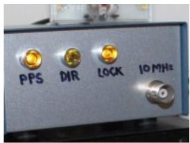
Here's a simple and easy single-chip 10.00000000MHz GPS-disciplined frequency reference, based 10MHz OCXO
