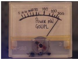
It's really simple to make a QRP power meter measuring RF output powers from a few mW up to half a
