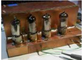
4. Mixer VFO using battery valves
