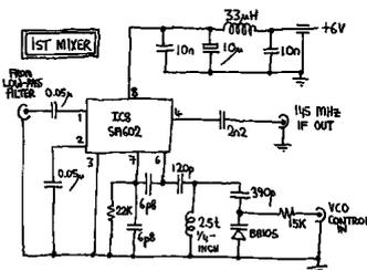
The best way to test this module is to connect the signal generator to its input, oscilloscope to the output, and manually control the VCO control voltage (see below).
