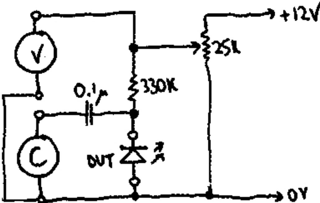
The results show a strong increase in capacitance as forward voltage is increased. NOTE: the voltages measured are at the wiper of the potentiometer, which is NOT now the voltage across the diode junction, since current is now flowing in the diode.
