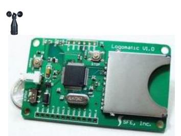
This wind logger project was designed to help a friend who wants to log wind speed for one year. It uses an inexpensive cup anemometer from Biral (see photo, left) available here in the UK. The anemometer contains a reed switch with rotating magnets which produce two switch closures per revolution of the cup assembly. It can be connected to produce a varying frequency output, whose frequency 0 - 100Hz corresponds to windspeeds of 0 - 40m/s.
