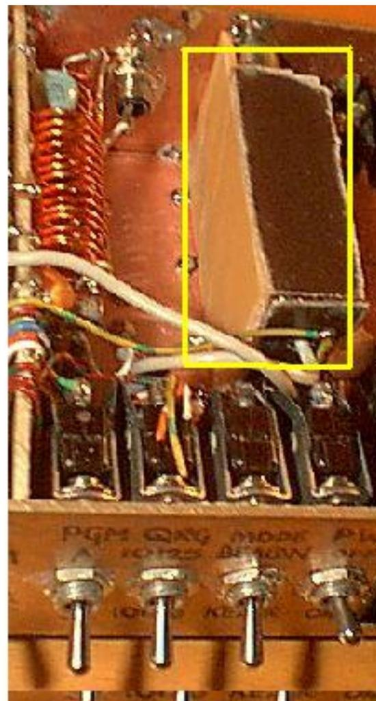
Next, I attempted to linearise the frequency shift (see the same-frequency 7'th and 8'th steps on the screenshots above). The lack of shift occurs when the shift changes from step 7 to 8. Therefore it is due to the 10K resistor in the resistor network being slightly off-value.
